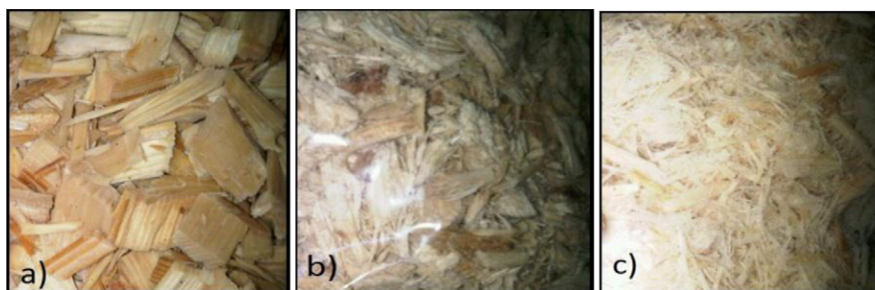
Fig. 1. (a) Original wood chip sample, (b) macerated wood chips, and (c) Very coarse pulp prepared using a KRK refiner.
